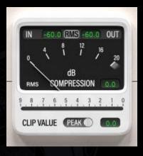
The dB COMPRESSION gain reduction meter main window shows the RMS (Root-Mean-Square) gain reduction applied to the signal as indicated by the ballistic needle.
