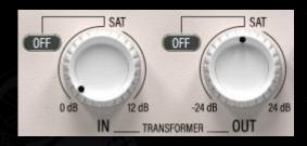
The T. IN and T. OUT gain knobs provide either pristine digitally clean or mojo infused transformer coupled amplifiers for adjusting gain pre and post
