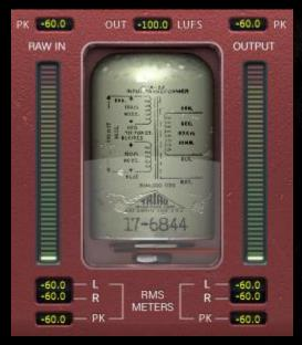
The metering shows several pieces of information including LUFS (Loudness Units relative to Full Scale) measurements, dBFS PK (decibels relative to full scale peak hold) measurements, and RMS / PEAK RMS (Root-Mean-Square) bar meters and measurements.
