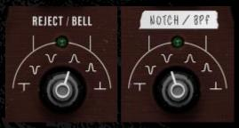
The switchable NOTCH/PEAK band filter selector allows for choice from three notch filters and three bandpass peak filters.
