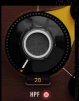
The HPF cutoff frequency knob sets the point from where the high pass filter starts working.
