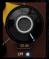
The LPF cutoff frequency knob sets the point from where the low pass filter starts working.
