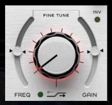
The High Shelf Selector knob allows for selection of one of a series of custom signature designed shelving filters.
