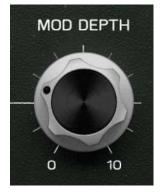
The Modulation Depth knob controls the LFO amplitude applied to the delay line, affecting the amount of pitch change. If this knob is at zero, the Modulation Rate by itself will not be able to affect the signal.
