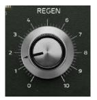
The REGEN knob controls the number of times a portion of the delayed signal is fed back into the beginning of the delay line. Setting this dial to a value of 8 or above will achieve a runaway effect. This effect requires caution because the output level will continue to increase to the point of internal clipping.
