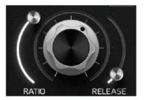
THRESHOLD sets the RMS level (not peak) from which the DKG circuit is triggered. RATIO: The amount of applied compression or downward expansion. RELEASE: It controls the recovery speed/time of compression (Duck) or downward expansion (KCUD and GATE).
