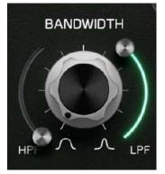
BANDWIDTH, HPF and LPF work together to form a single bandpass filter for the module's processed (wet) signal. The HPF and LPF set the filter's endpoints, while the BANDWIDTH knob fine-tunes it, tailoring the effect to sit perfectly in the mix.
