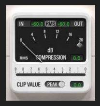
The dB COMPRESSION gain reduction meter main window shows the RMS (Root-Mean-Square) gain reduction applied to the signal as indicated by the ballistic needle.
