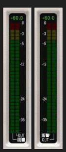
The LED meters shows peak and RMS input and output levels simultaneously, with RMS represented as the 'solid' continuously updated LED block in the main part of the meter, and with peak represented by the 'held' LED light, which will always appear above the RMS block.
