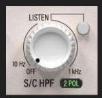
S/C HPF applies a high-pass filter to the detector circuit. This filter does not directly affect the sound of the processed signal. The slope of the HPF can be adjusted using the 1 POL / 2 POL switch to the right of the S/C HPF label. The 1 POL option
