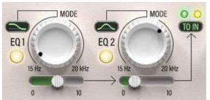
Two multi- functional EQ bands can be used to simultaneously alter the signal sent to the detector circuit (TO SC) and to alter the signal sent through the
