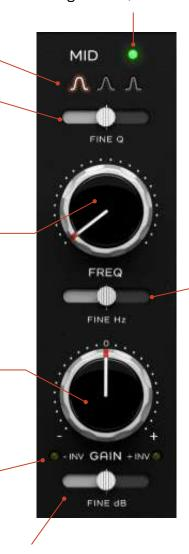
The FINE dB slider provides continuously variable gain adjustments.
