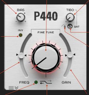
TIBO tightens the low end, resulting in an uncompromised sense of solidity and focus in the center of low imaging without altering the stereo image. When used in this manner, TIBO complements modern low-end stereo mixing techniques.
