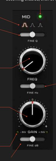
The FINE dB slider provides continuously variable gain adjustments.
