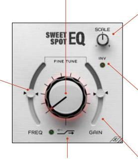
Each of the high/low arrows (found beside the on/off light) shifts the center point frequency and bends the curve in ways that are unique to each frequency selection. The SCALE simultaneously adjusts the GAIN and Fine-Tune settings for the LOW, MID, and HIGH bands. The middle position defaults to 0% scaling. You can increase boosts and cuts by turning the SCALE clockwise, or attenuate by turning it counterclockwise.
