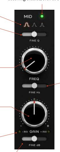
Resonance HUNT: While holding Mouse Right-Click on the FREQ knob or the FINE Hz slider, the Q gets tight and a medium boost is temporarily applied. This is a better approach than having a solo band mode, which can throw the ear off with too much abrupt contrast. Use Shift-Right Click for a temporary narrow notch band cut, instead.
