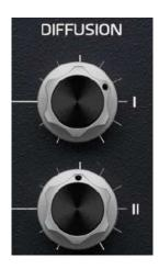
DIFFUSION is the scattering of an audible sound wave. The easiest way to understand diffusion is through an example. Consider the reflection of a click when it hits an irregularly shaped surface. A surface with high diffusion will cause the click to spread into a 'swoosh' of sound. A surface with less diffusion will cause the reflection to have a 'grainy' sound. A surface with low diffusion will cause the reflection to be an obvious series of clicks.
