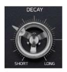
DECAY controls the amount of time it takes for the reverberant sound to fade away. This is implemented using a very smooth four stage decay process. The decay time is highly dependent on the selected PLATE SIZE. In addition to DECAY, the audible reverb tail can be heavily influenced by DAMPING. As it is with mechanical hardware, it is critical to experiment with different parameters while listening to and feeling how the audio is affected.
