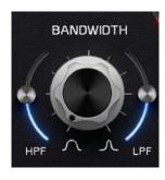
BANDWIDTH, HPF and LPF work together to form a single bandpass filter for the Plate REVERB signal. The HPF and LPF set the filter's endpoints, while the BANDWIDTH knob fine-tunes it, tailoring the effect to sit perfectly in the mix.
