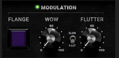
The 10% setting calibrates to the internal predefined values for each tape formula and speed. The sliders then adjust the effect based on percentages of this predefined baseline. Slow reflects typical tape machine tolerances. Setting it to 0% won't completely halt the tape machine's wow and flutter. You need to turn off the modulation circuit in this case.
