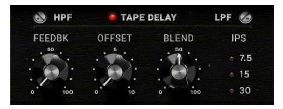
**HPF/LPF**: High-pass and low-pass filters that apply to the delayed tape signal.
