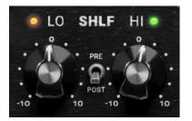
The POST position provides a way to refine the tonal balance after the tape has imparted its character. This is useful for restoring lost high frequencies, taming exaggerated harmonics, or simply making subtle tonal adjustments without affecting how the tape itself reacts to the signal.
