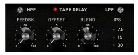
**HPF/LPF**: High-pass and low-pass filters that apply to the delayed tape signal.
